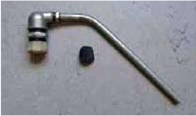
Retort made of a few inexpensive pieces of plumbing
