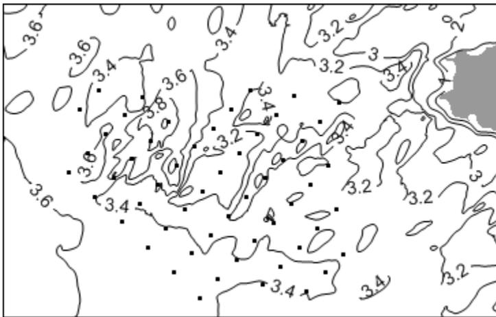
**Figure 4** The field distribution of saturated wave field of significant wave height at the wave farm 1. The contour unit is in m. Every black filled circle represents a wind turbine.
