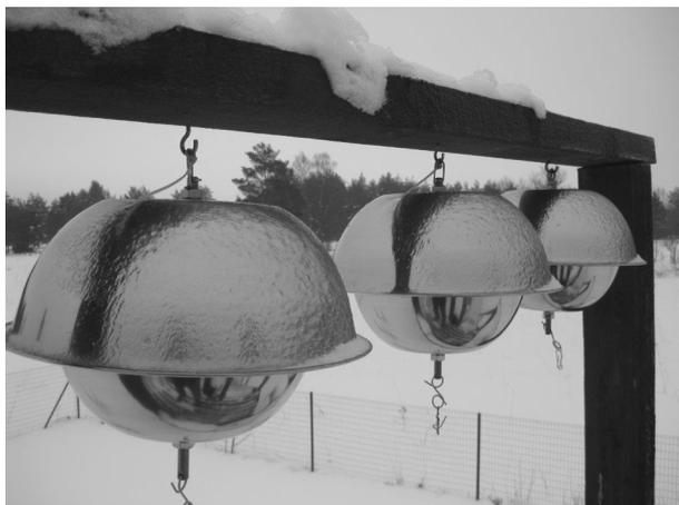
Fig. 1. Passive air samplers at the Lahemaa station.
