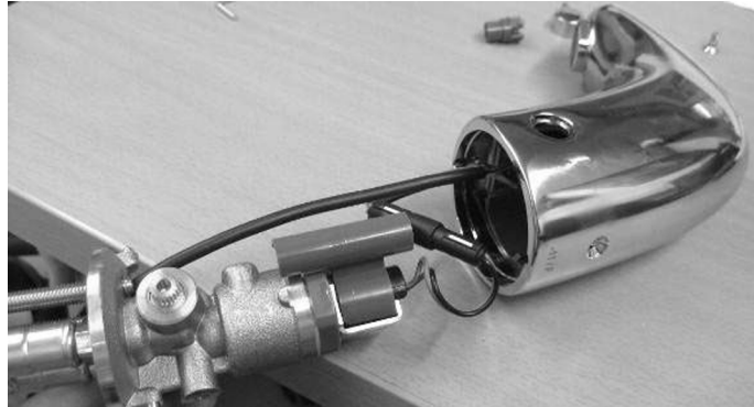
Fig. 1. Spout and internal components of the reference bathroom faucet.
