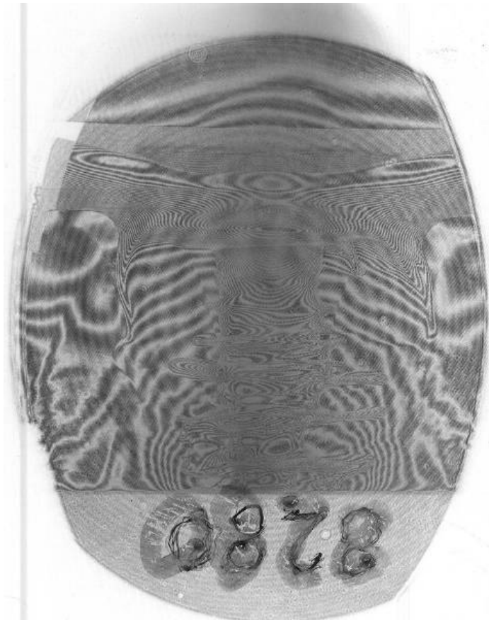
Figure 13. Typical interferogram taken at the moment close to maximal plasma compression
