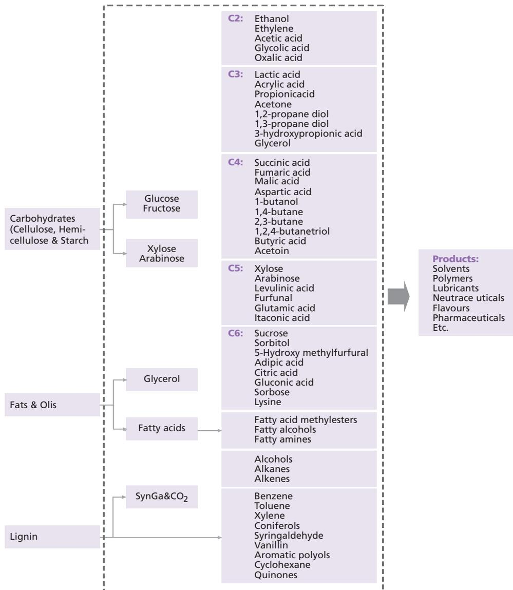
**Figure 7: Chemicals and products that can be obtained through biochemical processing of biomass**
