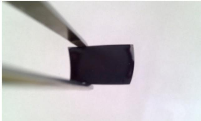
Figure 27 The most homogeneous ZnO/ZnO:In bilayer on polyimide substrate grown in laboratory of thin film chemical technologies by spray pyrolysis.
