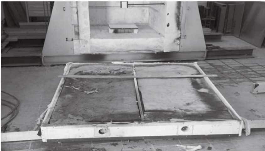
Figure 12. Local decomposition of the stone wool (left side) caused by vertical air flow through the construction during the fire test.
