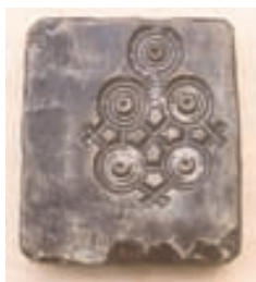
Moulds for casting simple tin ornaments
