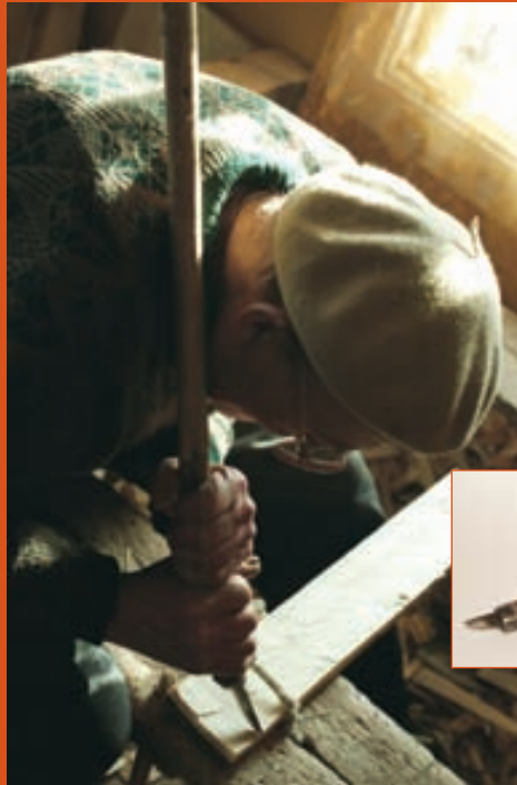
Cooper Elmar Reisenbuk from Avinurme cutting a croze with a grooving knife
