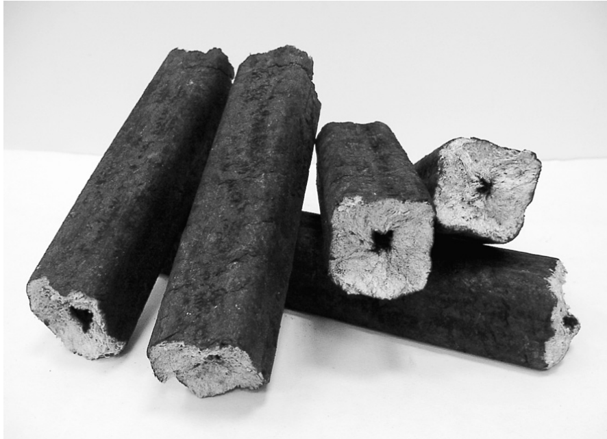
Joonis 3. Puitbrikett; W^t = 8-12\% , Q_a^t = 15-17 \text{ MJ/kg} , E^t = 0,7-0,9 \text{ MW}\cdot\text{h/m}^3 , A^k = 1-2\% , S^k < 0,05\% , N^k = <0,3\% , kloorisisaldus kuivaines Cl^k \leq 0,03\% Figure 3. Wood briquettes; W^t = 8-12\% , Q_a^t = 15-17 \text{ MJ/kg} , E^t = 0,7-0,9 \text{ MW}\cdot\text{h/m}^3 , A^k = 1-2\% , S^k < 0,05\% , N^k = <0,3\% , chlorine content in dry matter Cl^k \leq 0,03\%
