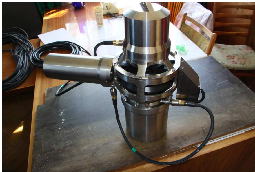
Figure 5.5: New Multi-spectral Volume Scattering Meter which was tested in Ukraine. Uus hajumismõõtmisteks loodud instrument, mida testiti Ukrainas.
