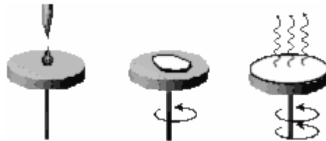
Fig. 26. Stages of the spin coating process: deposition of the sol, spin up, spin off and gelation by solvent evaporation.
