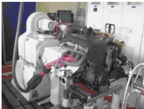
Joonis 1. Mootorite katsestend Dynas 3 LI250 ja katsetatav Audi A4 ADR mootor Figure 1. Engine test bench Dynas 3 LI250 and Audi A4 ADR engine
