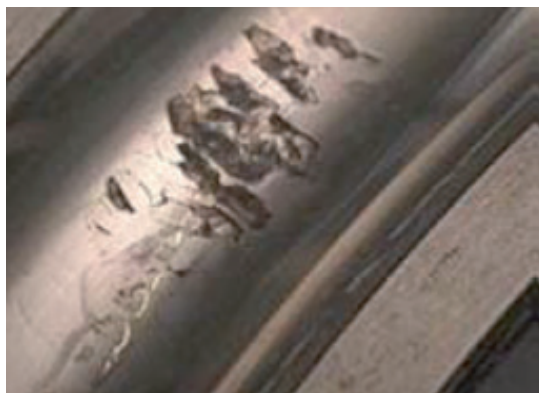
Joonis 2. Laagri pinnakihi vigastus (Lindh 2003). Figure 2. Flaking of the bearing (Lindh 2003).
