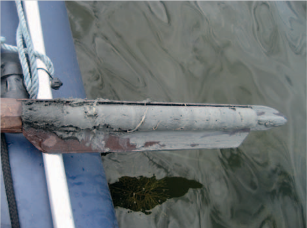
Photo 4.2.7.1. Sediment core from the Vööla meri. The sediment drill core is 50 cm long. Dark grey mud on the surface, followed by silt and in the bottom of the core by silt clay.
