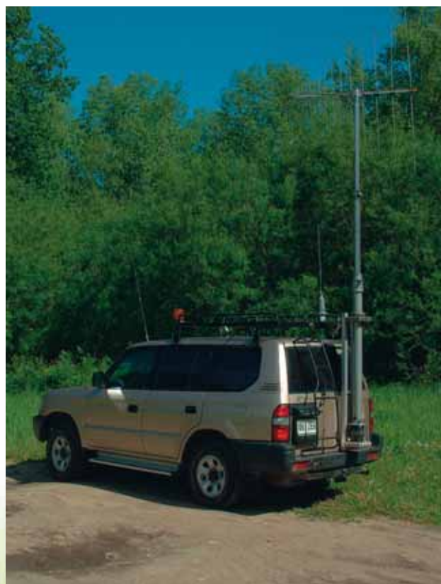
Mobile measuring station for detecting radio interferences and monitoring
