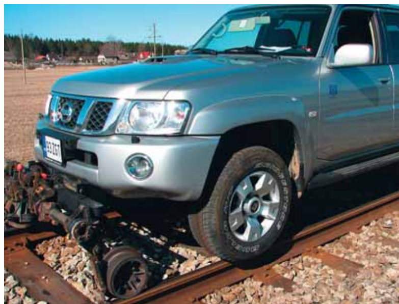
High-Rail vehicle - the control device of the railway infrastructure of the Technical Surveillance Authority
