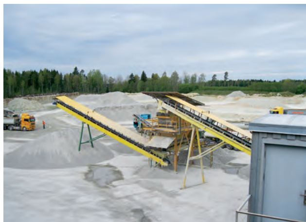
Crushing assembly in limestone quarry
