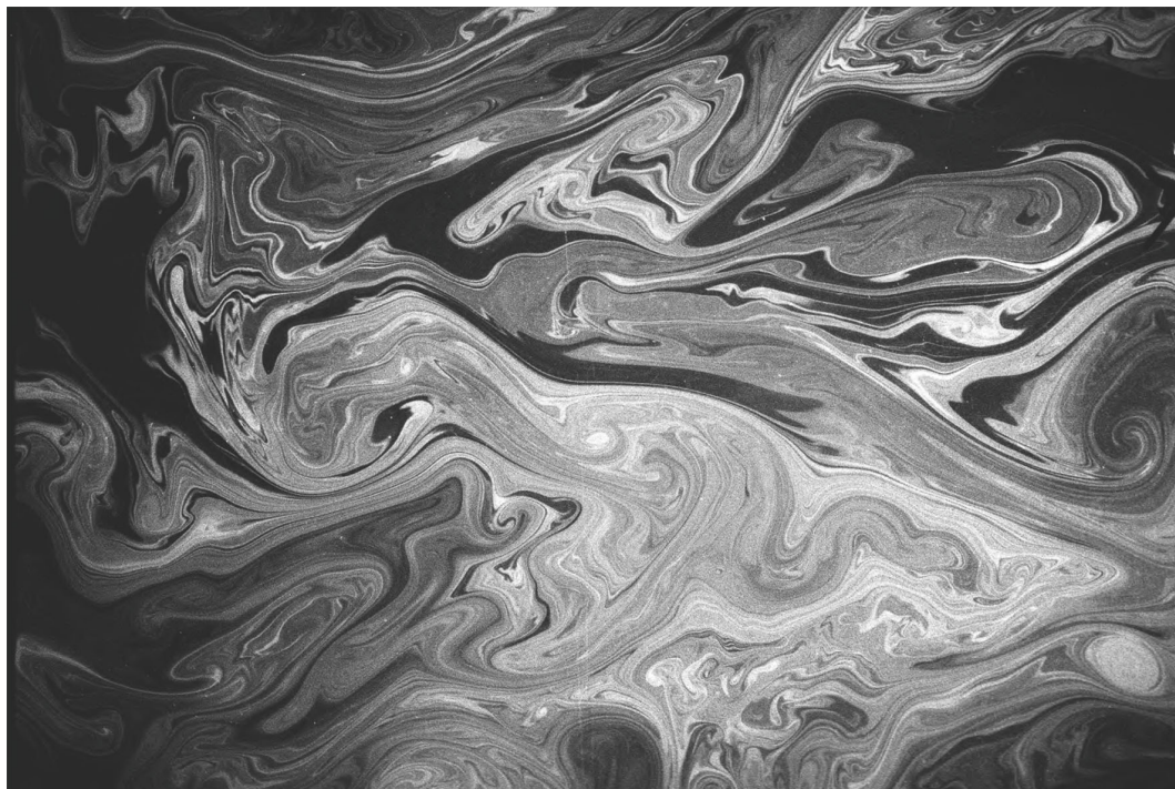
Fig. 1. A photo of the dye patterns recorded at the CORIOLIS tank in Grenoble in 1996 and used to obtain the graph in Fig. 2. A fluorescent dye has been injected into the quasi-two-dimensional high-vorticity flow in the tank; the dye was illuminated by a rotating laser and the patterns were periodically recorded by taking photos.
