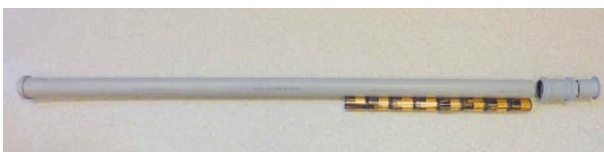
Fig. 2. A surface drifter constructed from a polyethylene tube and powered by eight standard D-size batteries used for the experiments in 2010–2011.
