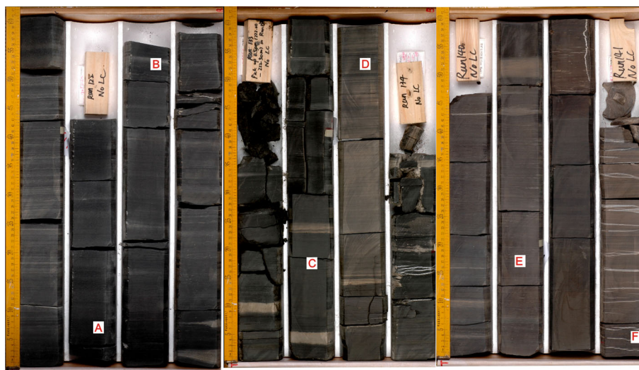
Fig. 2. Petrological characteristics of mudstone in the Qingshankou Formation, Songliao Basin: F – high-quality oil shale; C, D – medium-quality oil shale; A, E – low-quality oil shale; B – non-oil shale.
