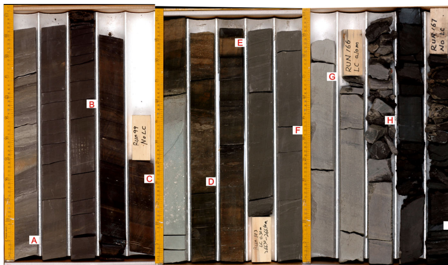
Fig. 3. Petrological characteristics of mudstone in the Huadian Basin. Letters correspond to the oil shale qualities and summarized chemical parameters presented in Table 2.
