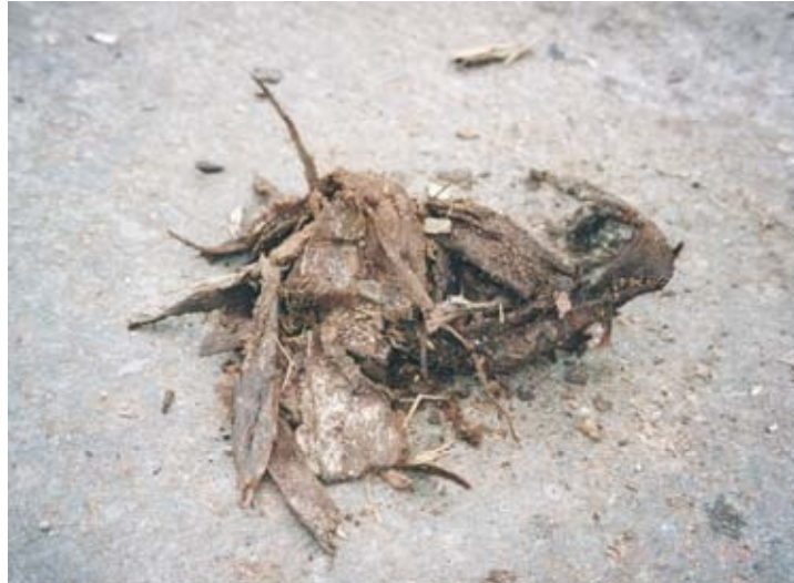
Joonis 1. Okaspuu (kuusk) koor; W^t = 50-55\% , Q_a^t = 7-8 \text{ MJ/kg} , A^k = 3-5\% Figure 1. Softwood (spruce) bark; W^t = 50-55\% , Q_a^t = 7-8 \text{ MJ/kg} , A^k = 3-5\%
