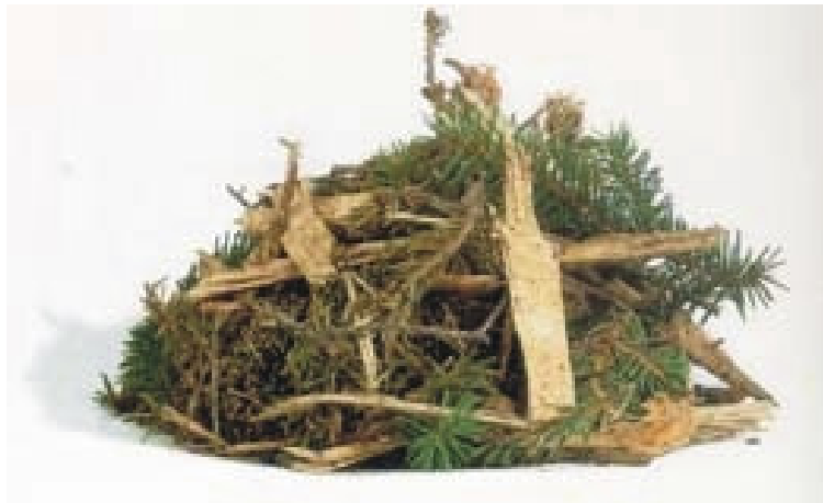
Joonis 2. Metsajäätmed; W^t = 45-60\% , Q_a^t = 6-9 \text{ MJ/kg} , A^k = 1-3\% Figure 2. Forest residue; W^t = 45-60\% , Q_a^t = 6-9 \text{ MJ/kg} , A^k = 1-3\%
