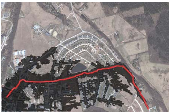
Illustration 5: red line presents the used path and the nodes evaluated by path planner are marked using dark area. Overall there was need to evaluate 25% of the aerial image for the path planning.
