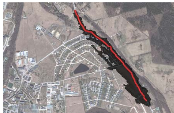
Illustration 4: red line presents the used path and the nodes evaluated by path planner are marked using dark area. Overall there was need to evaluate 7% of the aerial image for the path planning
