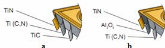
Fig. 1. Turning insert coating combinations
