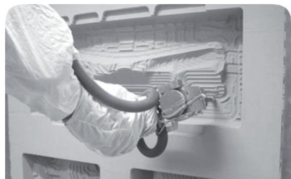
Fig. 1. Simtech's patternless casting milling robot. [1]
