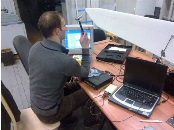
Fig. 3. Experimental modal analysis
