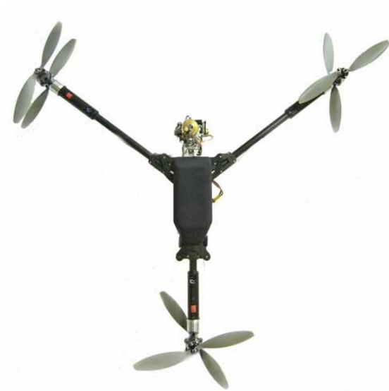
Fig. 11. Multirotor VTOL rotorcraft platform with gyrostabilized gimbal
