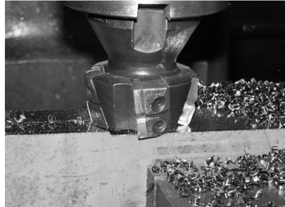
Fig. 2. Hard milling technological process of hardened abrasion-resistant sheet HARDOX 500, 46 \div 50 HRC [10].
