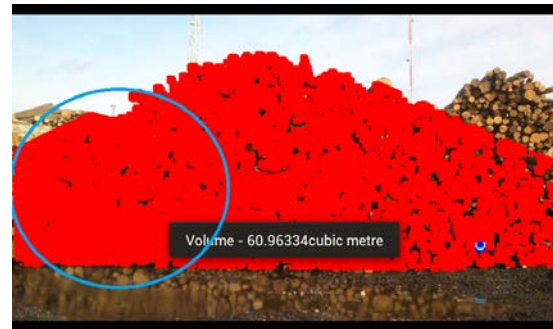
Fig. 13. Detecting the total area of the logs in pile.
