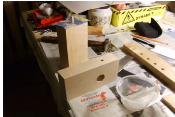
Fig. 7. Gluing of the shear strength test block
