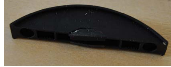
Figure 6. Failed Clamex P 15 specimen after bending test.
