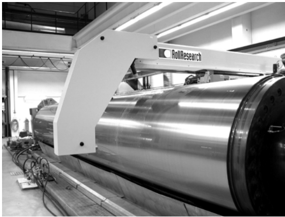
Fig. 1. Four point roll measuring device of a grinding machine. 1
