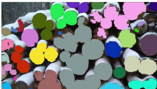
Fig. 9. The resulting image example. The pixels, which classified as a timber painted with random color.
