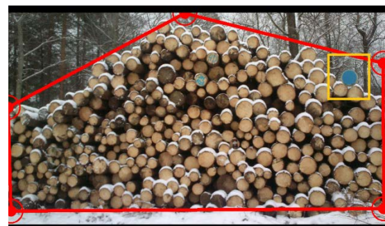
Fig. 11. Second screen for setting the ROI. The calibration standard is shown inside the box.
