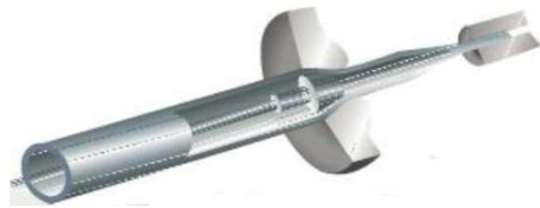
Fig. 1 Principle of tube drawing on mandrel
