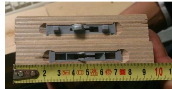
Figure 7. Failed Clamex P 10 specimen after tensile test
