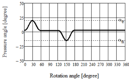
Fig. 10 Cam mechanism pressure angle, R_0 = 31mm and \varepsilon = -1.5mm
