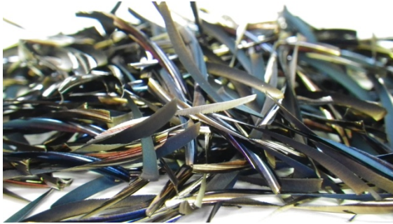
Fig. 1. Needle shape of chips after iMachining strategy
