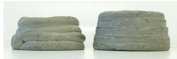
Fig. 5. Comparison of old and new result. The object on the right is printed with contour crafting.
