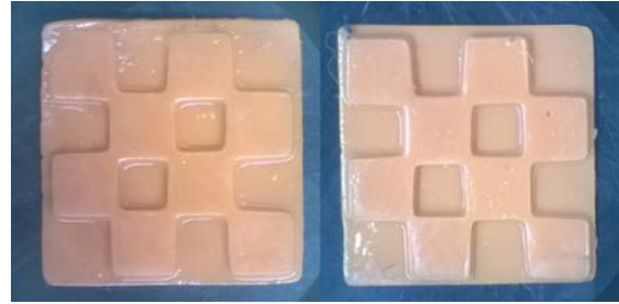
Fig. 9. Part created with white light on the left, with blue light on the right
