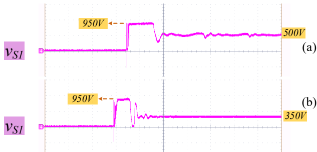
Figure 4.14 The overshoot voltage on the switches: (a) Proposed SSCBs, (b) Conventional SSCB in Fig. 4.1.
